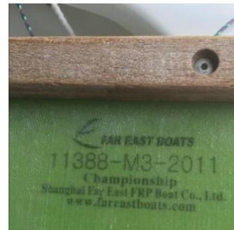
In this picture the Rudder serial number is 25mm down from the underside of the tiller. It's serial number is *FAR EAST 11350-M3-2011*
