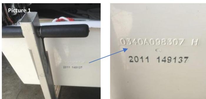
The ISAF number may be required at some events. The ISAF number is always on the starboard side of the thwart that the mast is stepped into. (Picture 2)
